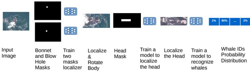
**Figure 1.** The overview of the method: First, two models are trained to localize the bonnet and the blow hole, respectively. Then, using these points, the body of the whale is localized and rotated so that the body has angle=0 with the  $x$  axis and the head is pointing east. After that, a model is trained to localize the head of the whale. Finally, a model is trained to produce a probability distribution over all possible whales.
