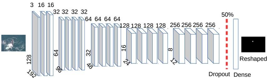
**Figure 5.** Localization architecture: the same architecture is used to localize the bonnet and blow hole, and later the head (in Section 6). The input of the architecture is an image of size  $128 \times 192$ . The output of the network is a layer with  $128 \times 192 = 24576$  possible classes. The output layer is simply a flattened mask and reshaping this layer gives us back the predict mask. The pixels with the highest intensities represent the location of the interest point.
