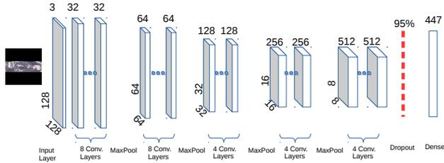
**Figure 7.** Recognition Architecture: the input to the network is an image showing the callosities of the whale. The output size is 447 corresponding to 447 unique whale IDs.
